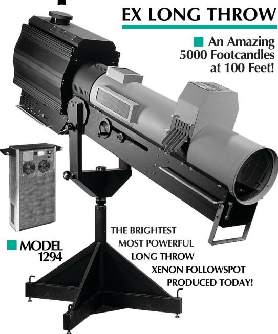
The Lycian 1294 SUPERARC XENON LONG THROW features a Dichroic "Cold Mirror" Reflector, Optical Grade Lenses, Nichrome Iris, Chopping Shutter, Fader, Quick Focus Knob and a Separate Electronic Switching Power Supply.
